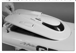
O 6. Remove the radio box cover from the hull by lifting it up using the tab at the rear of the cover.
