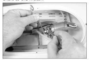
3. Remove the flex shaft by pulling it out of the stuffing box by the propeller.
