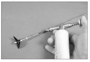
O 6. Reverse the previous steps to reinstall the flex drive. Check that there is a slight gap of 1/32-inch (1mm) between the stuffing box and propeller mount as shown. Also make sure the rudder mount is parallel to the rudder bracket when installed.
