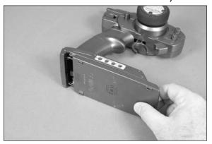
O 3. Install the four AA batteries in the battery holder. Match the polarity of the batteries to the molded markings in the battery holder.
