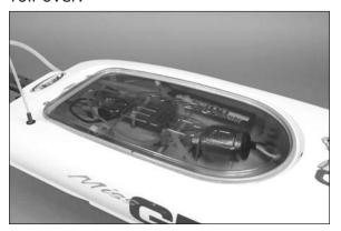
**Note**: The radio system is pre-bound at the factory but the 2.4GHz radio system may not bind correctly if the radio is adjacent to a large amount of metal such as an aluminum dock. Read the radio manual for binding details.
