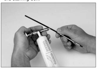
Note: Running the Miss Elam Brushless EP RTR in salt water could cause some parts to corrode. If you run the boat in salt water, rinse it thoroughly in fresh water after each use and lubricate the drive system.
