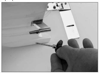
O 4. Slide the flex shaft out of the stuffing box.
