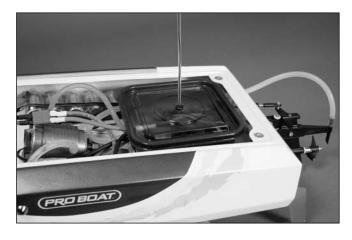
Turn the transmitter on, then turn on the receiver/ESC switch, checking for correct operation. The rudder control arm should move toward the front of the boat when right input is given. Conversely, when left input is given, the control arm should move toward the back of the boat.
