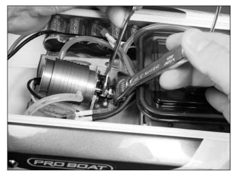
2. Loosen the 1.5mm setscrew connecting the universal joint to the drive shaft.
