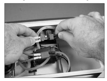
Attach the hook and loop material to the batteries and the battery boxes. Install two fully charged 7.2V Ni-MH battery packs into the hull.
