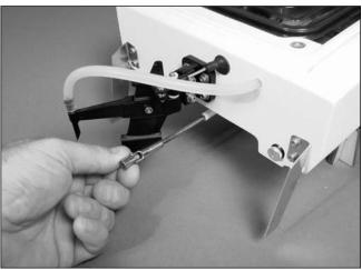
O 4. Lubricate the drive shaft with PRB0100 Water-Proof Marine Grease (see your local hobby shop). Reinstall the drive shaft in reverse order. Be sure to reinstall the nylon washer between the universal and the stuffing box.
