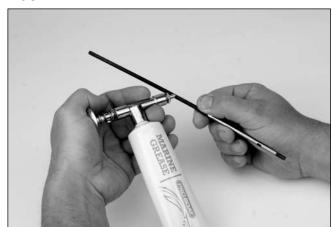
**Note**: Running the Blackjack 26 Brushless EP RTR in salt water could cause some parts to corrode. If you run the boat in salt water, rinse it thoroughly in fresh water after each use and lubricate the drive system.
