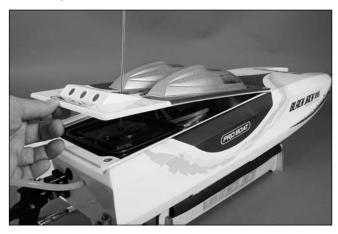
The Pro Boat water-cooled ESC comes pre-wired with a Deans-style connector. Use a 6-cell battery pack listed below for optimum performance.
