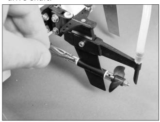
O 3. Move the rudder assembly and slide the drive shaft out of the stuffing box.
