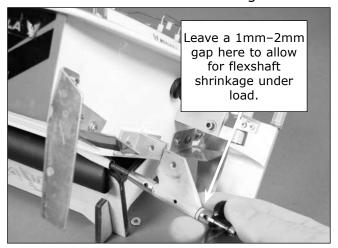
O 3. Lubricate the drive shaft with PRB0100 Water-Proof Marine Grease (see your local hobby shop). Reinstall the drive shaft in reverse order. Be sure to reinstall the nylon washer between the universal and the stuffing box.
