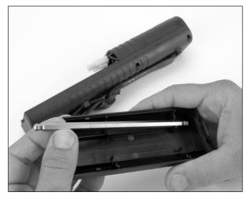
Step 2: Slide the starting wand (which is stored inside the battery cover) into the end of the starter, then replace the battery cover.
