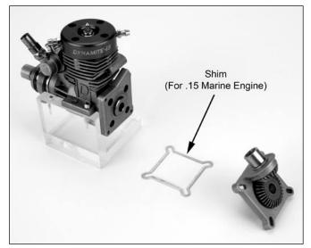
(.15 Marine Engine) Use the included shim plates between the backplate and the Tiger Drive main housing to create clearance for the starter shaft.
