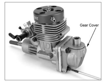
Step 5: Place the gear cover over the gears. Slide a 2.5mm lock washer, then a 2.5mm washer onto each of the 2.5  $\times$  10mm screws. Secure the gear cover using the 2.5  $\times$  10mm screws.
