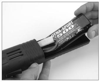
Step 1: Fully charge a 7.2V sub-C battery pack and install it in the starter as shown.
