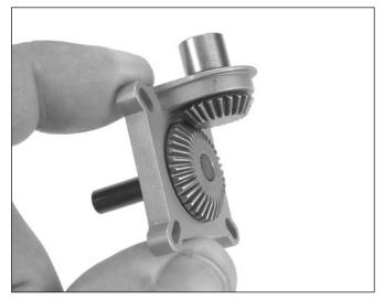
Step 3: Place the bronze washer behind the large bevel gear and insert them into the main Tiger Drive housing.
