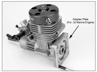
Step 2: Using the screws that previously mounted the pull-starter, attach the adapter plate to the engine. Use screw-locking compound on all screws.
