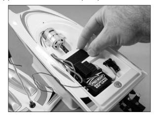
Attach the remaining hook and loop to the battery as shown.
