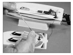
Slide the antenna cap onto the antenna tube to secure the wire in the tube.
