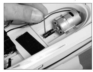
Loosen the 1.5mm setscrew connecting the universal joint to the drive shaft.
