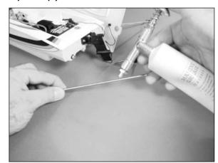
Lubricate the propeller shaft with PRB0100 Water-Proof Marine Grease (see your local hobby shop).
