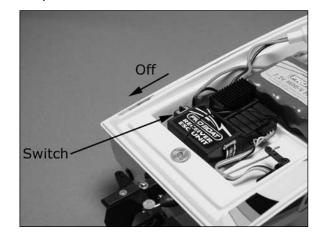
Plug the battery pack into the ESC.
