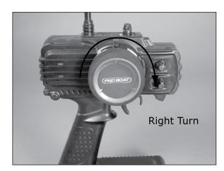
It may be necessary to adjust the rudder trim knob so the rudder is centered prior to operation. Use the Steering Trim (St. Trim) knob to center the rudder prior to operation. You may also need to finetune the steering trim to make sure the boat runs straight during operation. This can only be accomplished when operating the boat in the water and is detailed in a following section.
