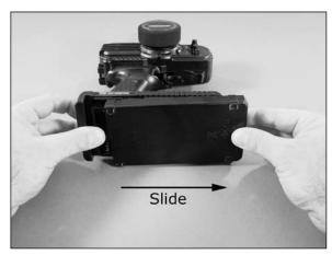
Install eight (8) AA batteries into the battery holder. Pay close attention to the correct direction of the positive (+) and negative (-) ends as marked in the tray.
