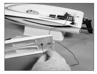
Slide the antenna wire into the antenna tube, pushing it through until it comes out the other end.
