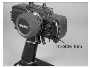
Give a small amount of throttle input by pulling the throttle trigger back to ensure the motor is working.
