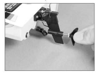
Move the rudder assembly to either the full left turn or full right turn and slide the drive shaft out of the stuffing box.
