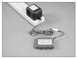
Change the battery for 1–2 hours before use. Never leave the battery pack charging for more than 2 hours or serious damage or fire may occur. When the battery is warm, disconnect from the charger.
