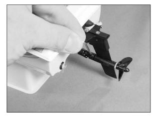
Carefully slide the propeller shaft from the rudder assembly and set aside.
