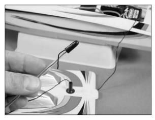
Push the antenna tube into the antenna mount.
