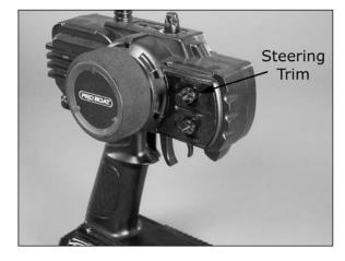
After you have completed checking your radio system, turn the Mini-C receiver off FIRST by sliding the switch to the "OFF" position. After the model has been turned off, turn off the transmitter.
