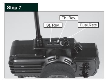
If you find the steering or throttle operate backwards as described in Step 6, you may need to switch the servo reversing as shown. In addition, you may also turn the dual rate dial down to reduce rudder travel in rough water conditions.
