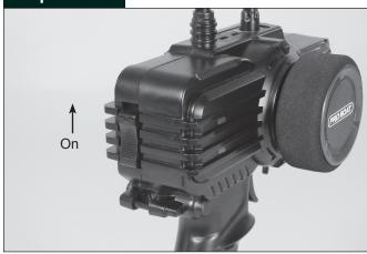
Always turn on the transmitter first by sliding the switch on the rear of the transmitter upwards. The small red and green lights on the side of the transmitter should both light up. If not, you need to check for low or incorrectly installed batteries.
