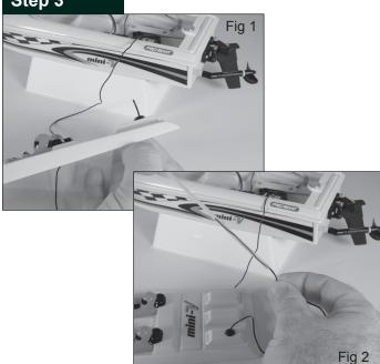
Push the antenna tube (Fig. 1) into the antenna mount. Insert the antenna wire through the antenna mount and into the antenna tube (Fig. 2) pushing it through until it comes out the other end.
