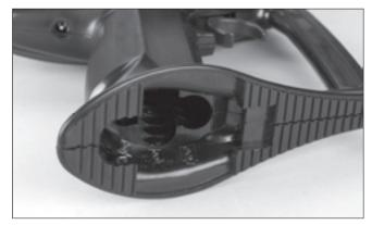
• 2. Remove the battery cover on the bottom of the transmitter.
