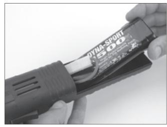
• I. Fully charge a 7.2V sub-C battery pack and install it in the starter as shown.
