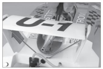
• 3. Use a 2.5mm Allen wrench to remove the tuned pipe mount as shown above.
