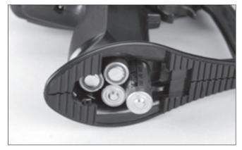
• 3. Install the "AA" batteries into the transmitter Be aware of the proper polarity when inserting the batteries.
