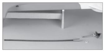
• 4. Carefully pull the ferrule away from the stuffing tube. You will need to pull at an angle to clear the aluminum strut.
