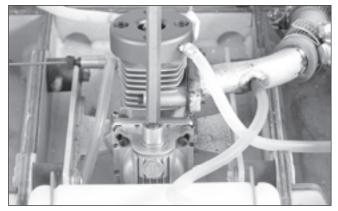
○ 3. Turn on your radio system and attach a fully charged glow igniter (DYN1925) to the glow plug. Insert the starting wand into the Tiger Drive and actuate the starting switch until the engine begins to run. If the engine does not start, place your index finger over the carburetor and actuate the starter until you see fuel enter the carburetor through the fuel line.
