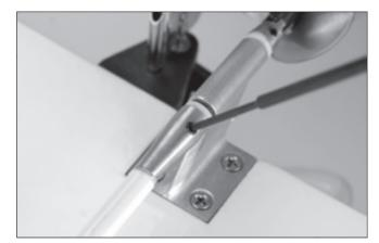
• 6. Carefully re-install the flex shaft and nylon bushing, making certain that you correctly tighten the collet nut. Next, re-install the drive shaft and propeller and tighten setscrews on the flats of the drive shaft.
