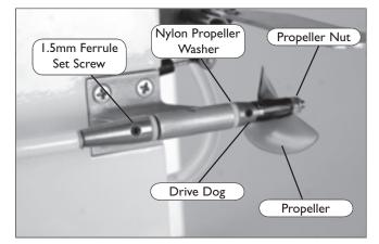
• I. Carefully note how the drive shaft and prop are presently installed. This is important so that when you have finished lubricating the drive shaft, you can correctly re-install the drive shaft.
