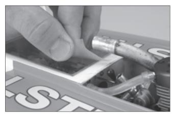
• 7. Re-install the battery holder back into the radio box and properly seal the radio box with clear tape. Failure to properly seal the radio box could result in damage to your radio equipment.
