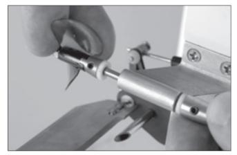
○ 2. Loosen and remove the 1.5mm setscrew that holds the propeller shaft. Remove the propeller and shaft from the aluminum strut.
