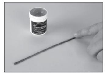
• 5. Liberally lubricate the entire length of the flex shaft with silicone cable grease as shown.
