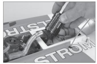
○ 6. Remove the dry cell battery holder from the radio box and unwrap the foam around the dry cell battery holder. Install 4 "AA" alkaline batteries into it as shown. Note the proper polarity. Wrap the battery box in foam.
