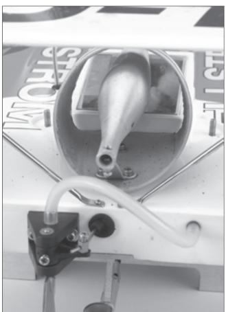
**O** 9. Re-install the tuned pipe mount.
