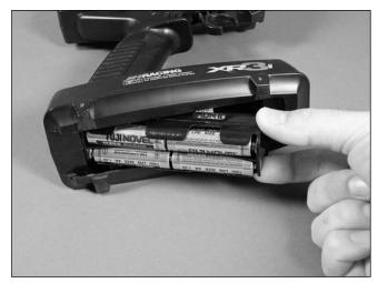
• 4. Insert the battery holder in the transmitter following the directions provided with the radio system.
