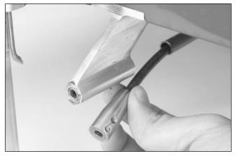
• 3. Remove the drive shaft flex cable. Replace the Teflon liner as needed.
