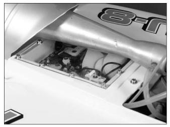
• 4. Plug the switch harness into both the receiver and the battery box following the instructions provided with the radio. Secure the radio box cover with the hex head screws.
