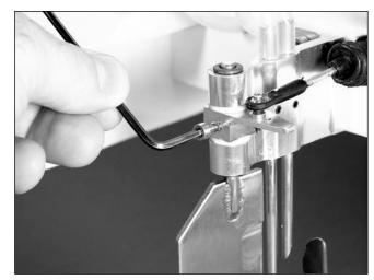
• 3. Find the flat spot on the rudder. Using the 2.5mm hex screw, tighten the hex screw on the flat spot as shown.
