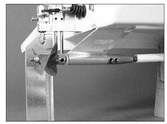
○ 5. Reassembly in reverse order. Make sure that the set screws are tightened down on the flat spots of the prop shaft. Also be certain to place a drop of threadlock on each set screw before re-tightening them.
