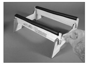
• 2. Secure the interlocking boat stand with medium thick CA or epoxy. Make certain you allow the CA or epoxy to fully cure before placing the boat on the stand.
