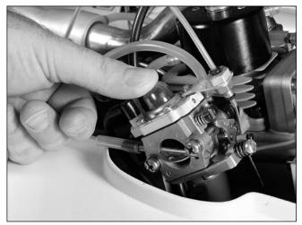
Press the priming bulb several times until it becomes filled with fuel. This is not necessary if the engine has recently been run.
