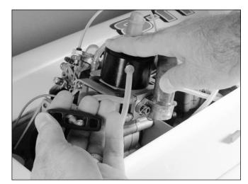
With an assistant holding the boat to the boat stand and bracing the engine with one hand, pull the starting cord briskly several times. Once the engine fires (begins to start), open the choke. Prolonged choking will flood the engine with fuel. See Section 15: Troubleshooting Guide to correct the flooding condition.
