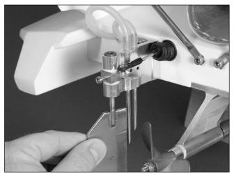
O 2. Carefully insert the rudder as shown.
