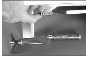
• 2. Loosen and remove the two 2.0mm set screws that secure the propeller shaft to the brass ferrule. Remove the prop drive dog and nylon washer.
