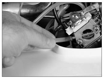
Close the choke by rotating the small yellow tubing extension. This is not necessary if the engine is warm.
