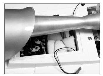
O 3. Wrap the battery holder in the foam provided. Secure the foam using a rubber band. Reinstall the battery holder into the radio compartment.
