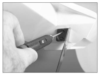
• 5. Carefully attach the turn fin onto the right sponson as shown and tighten the hex screws with a 3mm hex driver.
