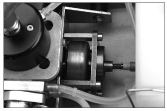
The centrifugal clutch automatically engages when the engine rpm is increased. Be sure that the idle speed adjustment is set low enough so that the propeller does not rotate at idle.
