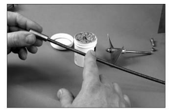
• 4. Lubricate the entire flex cable with waterproof grease as shown and then re-install the flex cable back through the liner and stuffing box and into the clutch.
