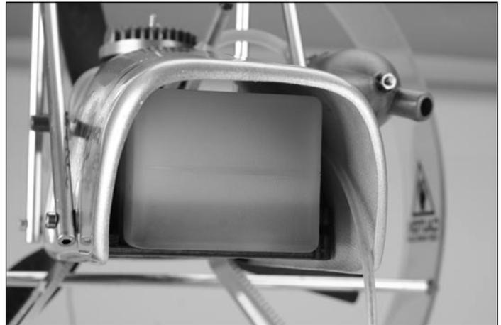
Checking the fuel level from rear of engine pod.
