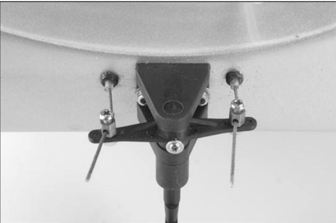
Rudder linkage setup.
