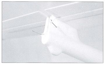
Insert the connector bolt of fin into the horizontal stabilizer and fuselage.
