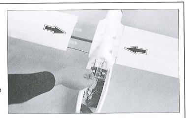
Fit the wings and the fuselage in place to avoid the wings loosening.
