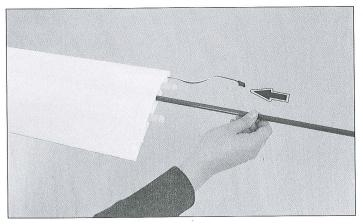
Put the aileron servo wire through the fuselage into the canopy.
