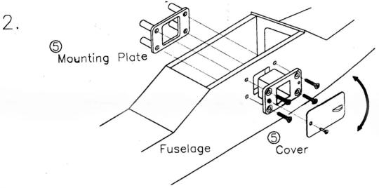
2/ Decide where the plug housing is to fit on the model and cut a hole to allow it to fit through the fuselage side. Attach the plug housing to the model using M3 x 15 self tapping screws through the fuselage side into the mounting plate (5). Attach the cover plate as shown with the M2 x 6 self tapping screw,. This screw should be tight enough to hold the cover plate in the correct position, but still allow it to be rotated to allow access to the glow plug.
