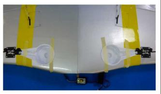
Turn on the power and set the gear down. Install the vacuum-formed mounts for wheels on the main wing and secure them in place with instant glue.
