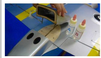
Insert the wing bolts and washers through the venting. Try to the fit the vent onto the main wing with the wing bolts into the bolt holes.
