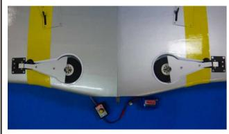
Assemble the gear covers to the gear mounts. Secure the axles to the main gear with M3x4 screws. Install the wheels and collars.
