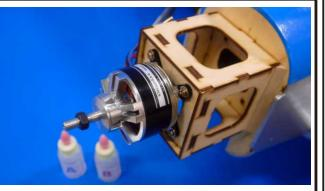
Use Epoxy to secure the motor mount on the fuselage and reinforcing blocks on two sides of moor mount.
