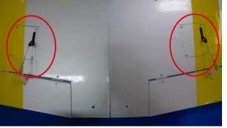
If use Y-harness on the flap, please install the left wing and right wing servos at the same side. If want to use mixer on the radio, the location of both servos must be on different side.
