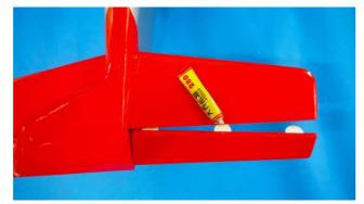
Use Super glue to secure the hinges insides the hinges slot of elevator. Also use Super glue to secure the half of hinges to the horizontal.
