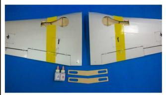
Spread generous amount of 30-min epoxy to the top and bottom of wing joiners, and wing root. Insert the wing joiners to the left and right main wing for securing both main wing together.
