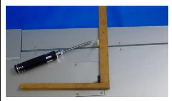
Place the triangle rule along the servo arm to the trailing edge for setting the location for installing the control horn on the aileron. Use 1.5mm hand driller to drill holes for the control horn. Place the control horn in position and the strap on its back and secure with M2x25mm screws.
