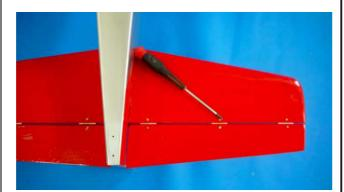
Use 2x15mm tapping screws to secure the hinges. Use side-cutter to remove extra length of screws.
