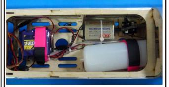
Use Velcro tape to secure the tank and receiver inside in fuselage.
