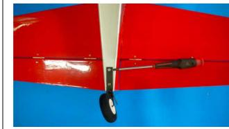
Secure the tail wheel to the tail gear. Use M3x10 tapping screws to secure the tail gear mount to the tail.
