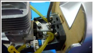
Connect the throttle rod with ball-end.
