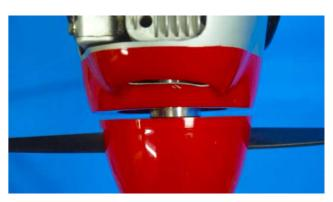
Assemble the spinner with propeller. Install the spinner to the motor. Please keep the distant between spinner and cowl around 2mm.
