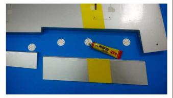
Spread some Super Glue on the top and bottom one-half of each hinge. Insert the hinges into the main wing until the hinge line is even with the trailing edge of the main wing.
