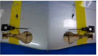
Place the main wing upside down. Try to find the Y-harness from the main gear mount. Plug the Y-harness and apply some transparent tape around the plug. Assemble the retracts on the main wing with M3x12 tapping screws.
