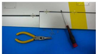
Spread some Super Glue to the remaining half of each hinge and place the aileron and flap onto the main wing. Secure the hinges with 2x15mm tapping screws. If the end of the screw is too long, use side-cutter to trim the end.
