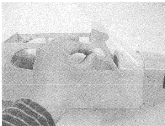
Try to place the front window on the fuselage. When satisfy the location, use tape to secure the front window in place.
