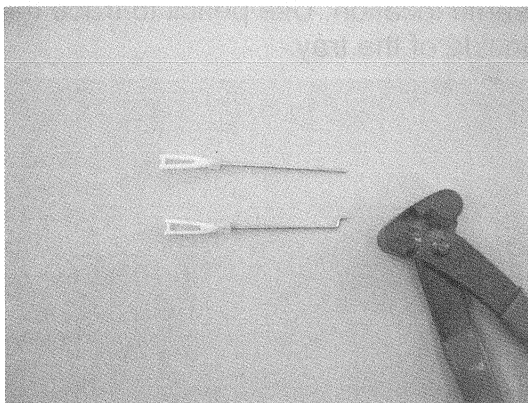
Use Z-bender to make a Z on one end of the aileron rod.
