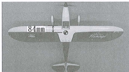
The recommended Center of Gravity location is 84mm back from the leading edge.
