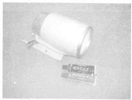
用AB膠將動力組之保麗龍外罩黏合. Use epoxy to glue the foam cover on the duct fan.
