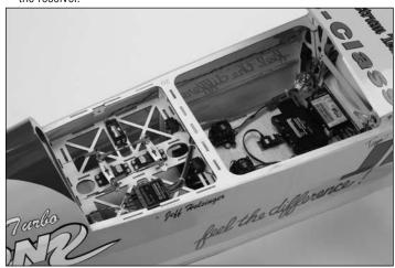
2. Mount the switch on the side of your aircraft and insert the switch plug in the port in the main unit marked SWITCH.
