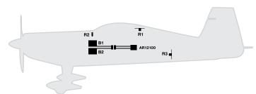
40% aerobatic plane with dual LiPo batteries, dual regulators and four remote receivers
