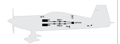
• Jet with dual LiPo batteries, dual regulators and four remote receivers
