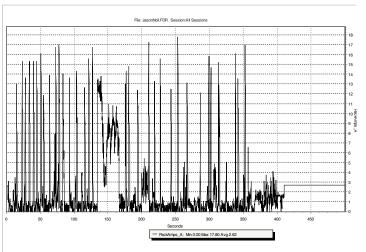
In the example above, the average current was 2.62 amps, which calculates to 435mAh per 10 minutes (typical flight length). It's recommended that only 60% of the available capacity be used to ensure plenty of reserve battery capacity. In this example using two 4000mAh batteries (8000mAh total capacity) x 60%= 4800mAh (available usable capacity) divided by the capacity used per 10-minute flight, 435mAh would allow up to 11 flights, of 10 minutes each.
