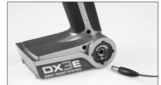
Optional NiMH 1.2-volt AA rechargeable batteries (SPM9525) can also be used. If rechargeable batteries are used, they can be conveniently charged without removing them from the transmitter by using the charge jack located on the back side of the transmitters base.
