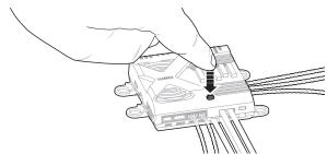
**NOTICE:** If using a bind plug, remove after binding to prevent the system from entering bind mode the next time the power is turned on.
