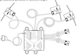
Using foam or thick double-sided foam tape and tie wraps, secure the main PowerSafe unit in the position where you would normally mount the receiver.
