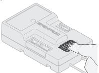
can come in handy if the receiver needs to be mounted in a location that is difficult to access, in which case a servo extension may be used for binding. If using a bind plug, remove after binding to prevent the system from entering bind mode the next time the power is turned on.
