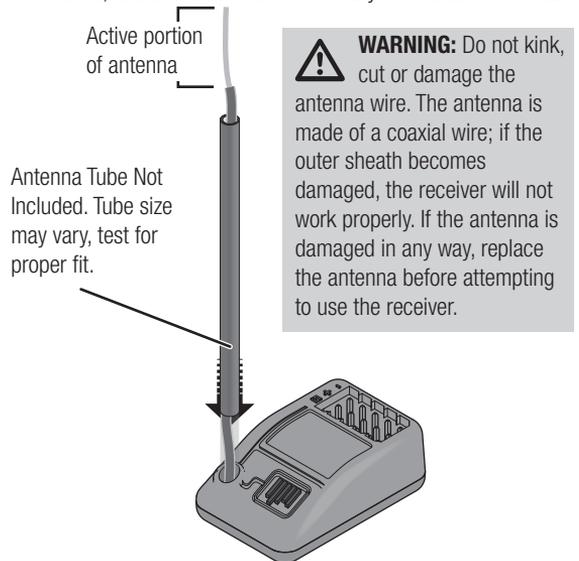
The case of the receiver can accept an antenna tube directly, making optimal antenna placement easy (antenna tube not included).
