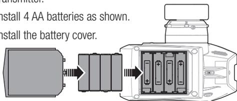
**CAUTION:** NEVER remove the transmitter batteries while the model is powered on. Loss of model control, damage or injury may occur.
