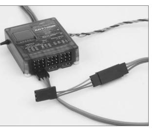
The AR7100/AR7100R feature two types of fail-safe: SmartSafe<sup>™</sup> and Preset Failsafe.
