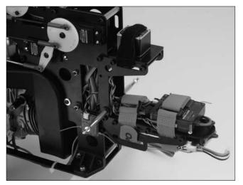
• Mount the Receiver unit in the position recommended by the helicopter manufacturer. Foam or thick double-sided tape is recommended to isolate the receiver from vibration.
