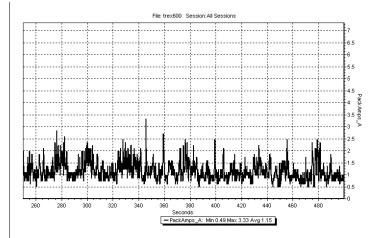
In the above example the average current was 1.15 amps, which calculates to 153mAh per 8 minutes (typical flight length). It's recommended that only 60% of the available capacity be used to ensure plenty of reserve battery capacity. In this example using 2000mAh batteries 2000 x 60% = 1200mAh (available usable capacity) divided by the capacity used per 8 minute flight, 153mAh would allow up to 7 flights of 8 minutes each.
