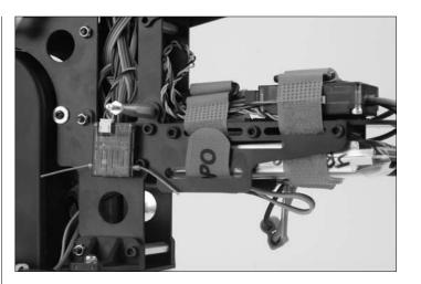
• If using the RevLimit Limiter (AR7100R only) mount the rpm sensor and bracket to the backplate under two backplate screws of your engine as shown.
