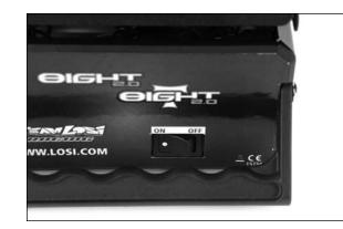
Press down on the rear of the chassis to engage the starter box wheel to the flywheel. After the engine starts, release the chassis. The vehicle will be able to sit on the starter box fixtures and idle without interference.
