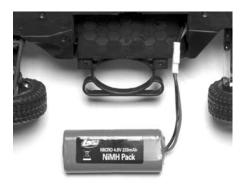
2. Plug the AC charger into the proper wall receptacle (110V - US version). Plug the battery pack into the charger and let it charge for 1 hour for the first time. Charge for 1 hour thereafter for a full charge. Battery charged for over 1 hour may cause an overcharge.
