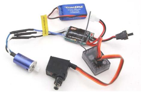
An example of connection for LOSB9595 Brushless Combo with the motor and battery connected.
