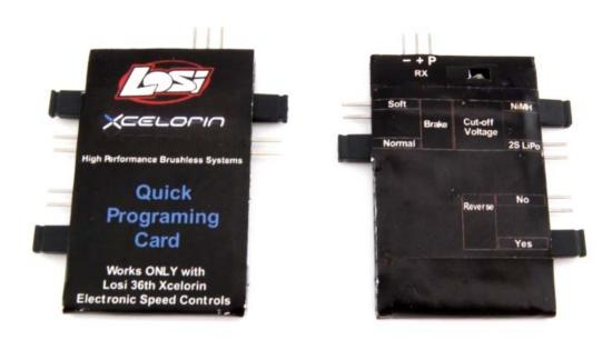
The supplied Quick Programming Card (QPC) is used to setup the Electronic Speed Control to your operating requirements.
