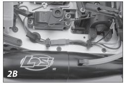
Using the charger of you choice, follow the manufactures instructions and charge the receiver battery pack mounted in the chassis. (fig. 2A). After the pack has been charged plug the battery into the switch harness (fig. 2B).
