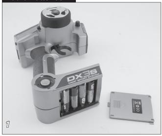
Install the 4 AA-size alkaline batteries in the transmitter making sure the positive (+) and (-) negative ends are oriented correctly.
