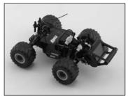
Plug in the battery lead into the speed controller lead and replace the body. Secure the body with the included body clips.
