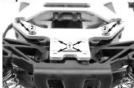
Remove 4 chassis screws (1). Loosen chassis screws (2) enough to allow the bumper to slide out from under the chassis plate. NOTE: If you are rebuilding the front diff, skip to step 6.
