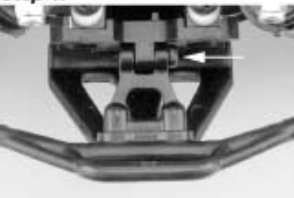
Remove upper bumper mount screw.
