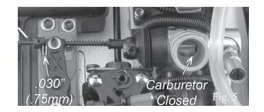
7. Watch the throttle linkage as the transmitter trigger is slowly moved to the full throttle position. Adjust the throttle EPA on the transmitter so that the carburetor only opens 90-95% of its total travel (Fig. 6).
