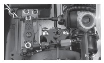
The throttle portion of the linkage adjustment is now complete. Do NOT proceed if the above test does not work, repeat the procedure if necessary.
