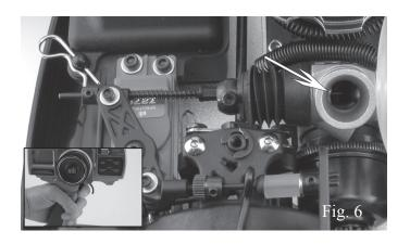
8.To ensure that the EPA or Travel Adjustment is set correctly, apply full throttle on the radio and gently pull on the throttle linkage rod. There should be at least 0.030" (0.75mm) of additional travel (Fig. 7).
