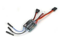
The ESC has connectors installed and ready for your use. The motor will connect to the ESC Motor wires by matching colors, Blue to Blue, White to White and Black to Black. Doing this the motor will run the proper direction for your Losi Micro Vehicle. Should you need the motor to operate in the opposite direction just disconnect any two of the connectors and reconnect in reverse fashion.
