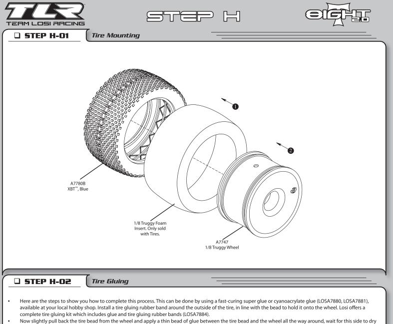
Now slightly pull back the tire bead from the wheel and apply a thin bead of glue between the tire bead and the wheel all the way around, wait for this side to c
