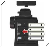
CAUTION: NEVER remove the transmitter batteries while the vehicle is powered ON, as loss of control, property damage or injury may result.
